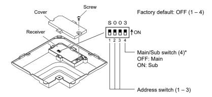
\* When using the infrared remote controller and the wired remote controller in combination, set the wired remote controller to [Main].
