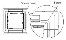
3 Place a hand on both the right and left convex parts of the corner cover to remove it.
